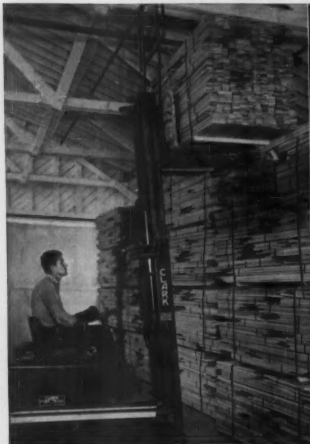
Unitizing of random length hardwood flooring permits quick and easy handling for storage. Idea 531
